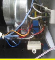
Crimp connectors 3 mm from housing or is housing 850 degree GWT approved?Can pass.
